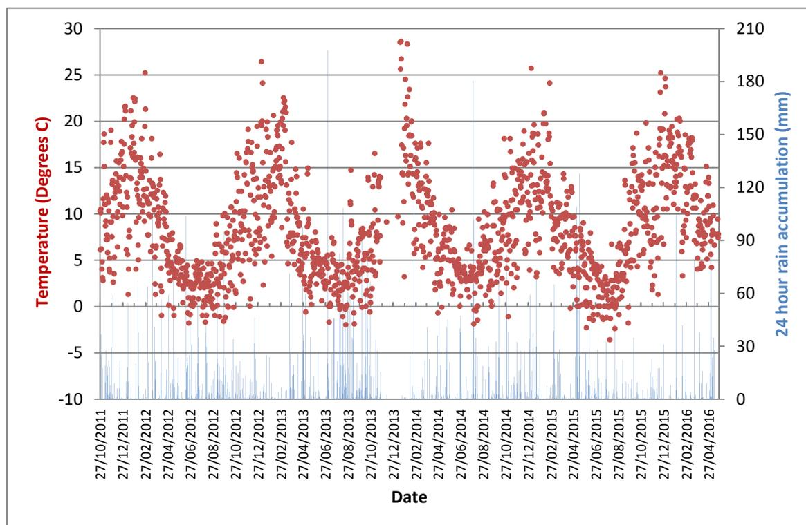
**Figure 2.** Maximum daily temperatures at 1286m above sea level on Cradle Plateau, as measured at 2m above ground level (red dots) and 24 hour rain accumulation (blue bars). This Automated Weather Station commenced operation in October 2011. Note the five days over 25°C in January 2014 during one of the most extreme high altitude heat waves on record in South Eastern Australia.
