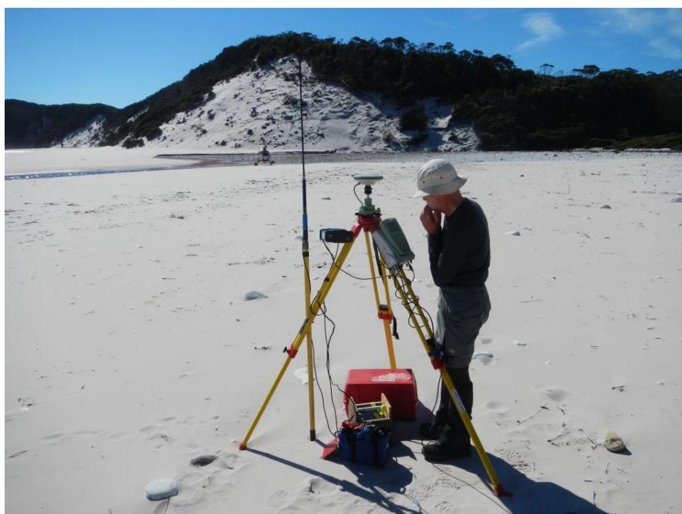
Monitoring coastal sand erosion and accretion requires accurate measurement. Here, surveyor Nick Bowden establishes a temporary survey base station to provide an accurate reference for a survey transect across the face of this beach-backing dune.
