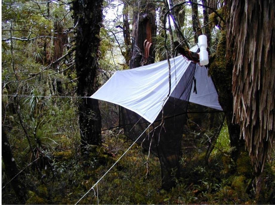
Malaise traps are used to collect flying insects. Insects fly into the black mesh barrier hanging down from the apex of the white canopy sheet. They then crawl upwards towards the sunlight and enter a collecting bottle where they fall into the alcohol-filled container. The trap was set up at 800m on Mt Weld.
